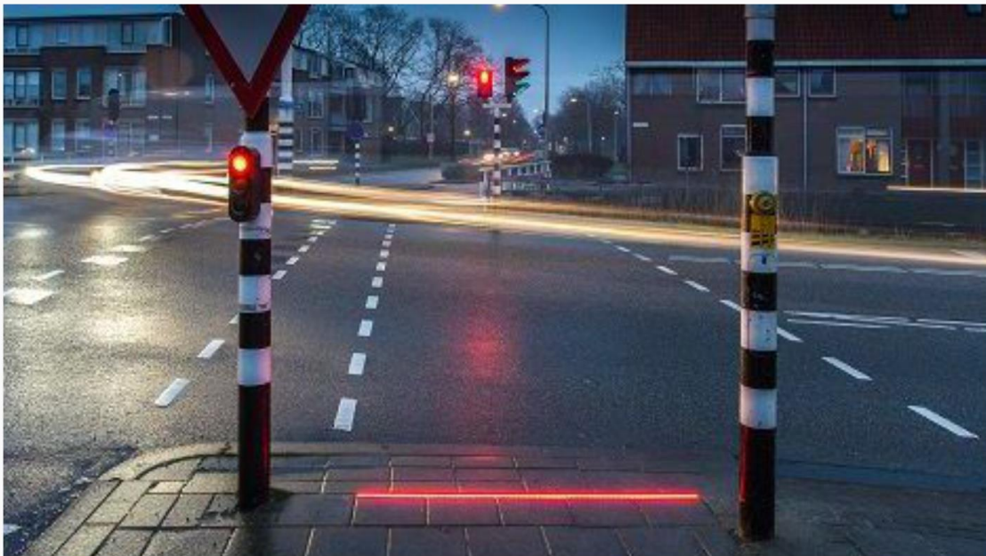
Figure 31. City of Bodegraven, (The Netherlands) LED light strips on the sidewalk synchronized with traffic signals 218
