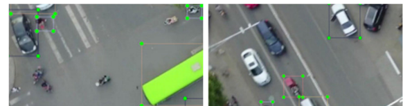
FIGURE 29. Amplification of Figure 27 showing targets (cars and motorcycles) that are perfectly identifiable and not labelled in the dataset.
