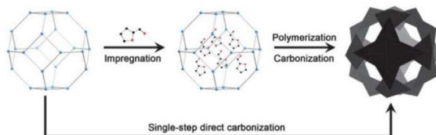
Figure 4. Schematic representation of porous carbons from MOF with furfuryl alcohol as an additional carbon source and direct carbonization of MOFs. Reproduced from ref. [65]. Copyright © (2013) with permission from the Royal Society of Chemistry.
