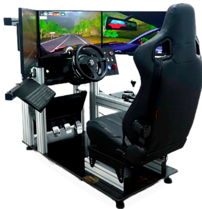
Figure 1. Simescar LITE driving simulator (SIMUMAK) used in the study.
