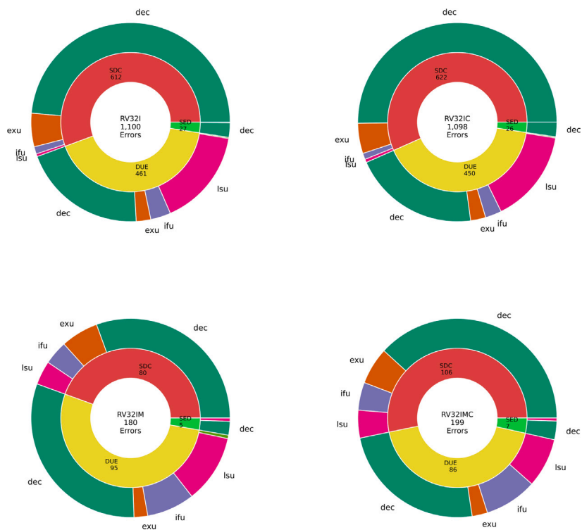
Fig. 12. CCSDS - Conditional probability of originating bitflip unit given an error category (4 ISAs).
