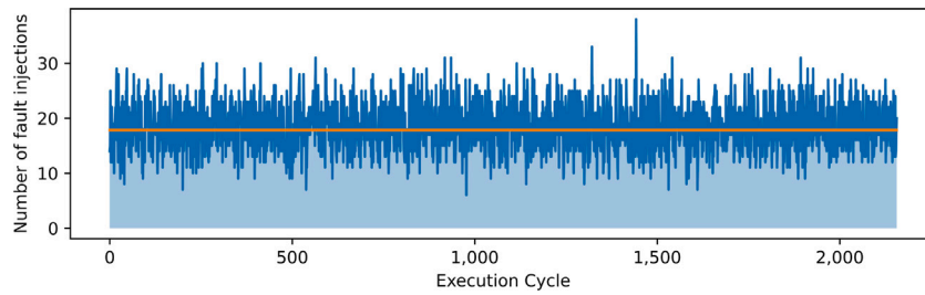
Fig. 5. Injections per cycle (blue) and average injections per cycle (orange) for the DOT algorithm. (For interpretation of the references to color in this figure legend, the reader is referred to the web version of this article.)
