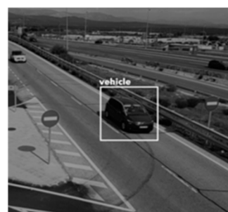
Figure 7. Vehicle detection using the “heavy” model from a computer, using the same image as the previous example.
