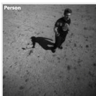
Figure 5. Identification of people in a frame from overhead view using the person detection model on Arduino Portenta boards.
