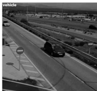
Figure 6. Vehicle detection using the “lightweight” model from the Arduino Portenta board.
