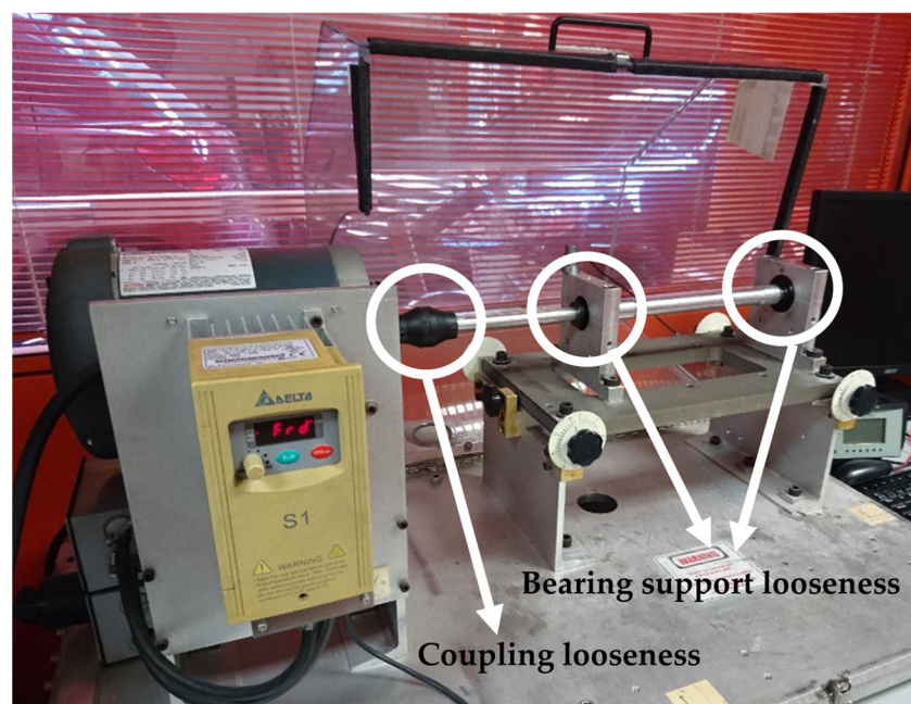
Figure 1. Experimental test bench used for vibration acquisition, showing the motor, mechanical coupling, rotating shaft, bearing supports, and accelerometer mounted on the bearing housing closest to the motor.
