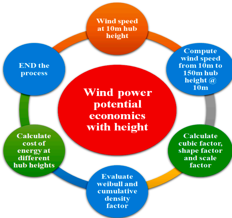
Fig. 2. Economic cost study of wind turbine installation at varying tower height using proposed wind power generating potential assessment.
