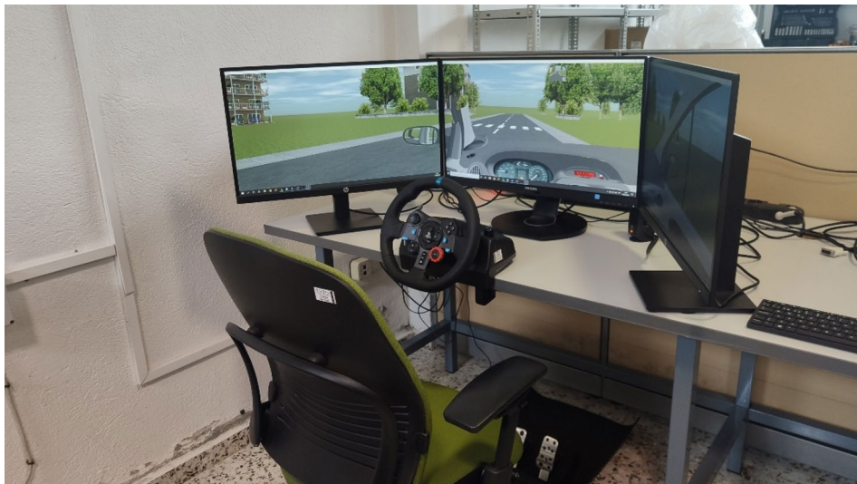
Fig. 1. Driving simulator setup used in the experiments, consisting of a steering wheel with pedals, three monitors displaying the virtual driving environment, and a participant’s chair. Driving simulator setup used in the study. The system includes a steering wheel with pedals, three monitors providing a wide field of view of the virtual driving environment, and a participant’s chair positioned in front of the workstation. This setup was used to conduct all trials and to record participants’ driving performance under controlled conditions.
