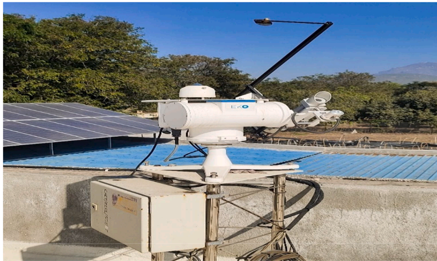
Fig. 8. Sun tracking system with pyranimeter and pyrhemliometer.
