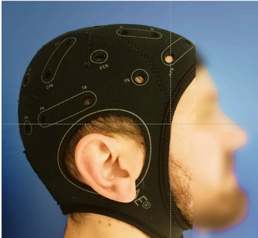
Figure 6: Neoprene cap for HD- tDCS stimulation. The cap has holes to place electrodes following the 10/20 classification system for EEG. Please click here to view a larger version of this figure.
