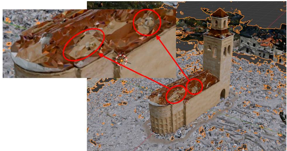
Figure 6. Rooftop with prediction errors. A possible solution would be to increase the dataset to include a bird’s-eye view, so the model can observe the rooftop and predict its point positions [X, Y, Z] . The image provides an overview of the building’s roofs, with a zoomed-in view on the left side. The circles indicate areas that are difficult to reconstruct due to being hidden from street-level perspective images, which do not capture the roof. Figure created by the authors.
