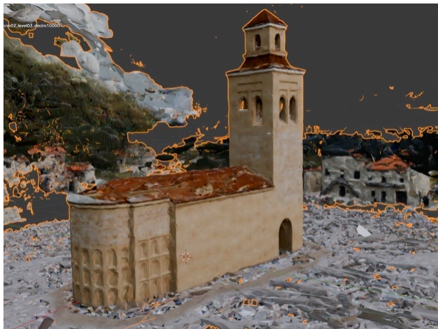
Figure 5. SuGaR output mesh viewed in Blender 4.0 of church 01 after “cleanup” in experiment 2. This image illustrates the type of mesh geometry that SuGaR’s outputs when using Mip-splatting’s .ply output as input. This .obj output file exhibits meshes (and therefore a point cloud) with significant noise, and they had to be “cleaned” by hand for the 3D model to be observed. Refinement set to 15,000 iterations and polygon count to one million with one Gaussian per triangle. Figure created by the authors.
