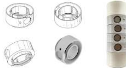
Fig. 1. The AMBER device. On the left side of the image, the sketch of the layout of the sensory cylinder modules of the device seen from various angles and the 3D layout. On the right side, the device prototype made up with four modules, each with one RGB LED and one FSR.
