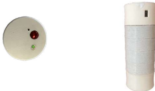
Figure 4.9: Button and hole for the USB-C charging connection.
